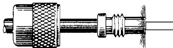
Figure 5 - Folding the shield braid strands over the end of the reducer.
